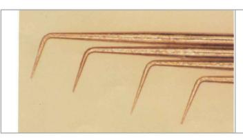
We have successfully established tip bending process for probe card pins.
